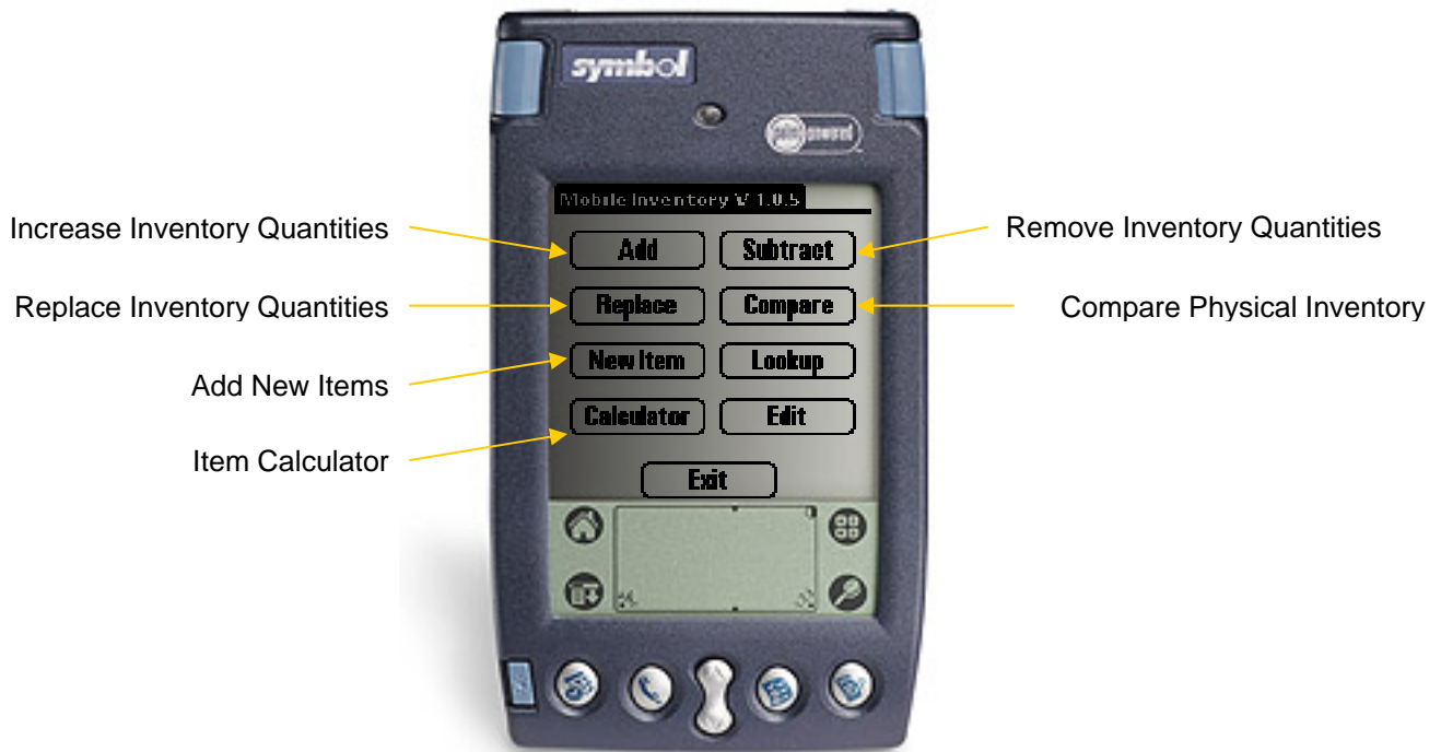
Figure 3.2 Scanner Main Menu
