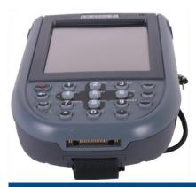
Also, the charging/interface cable plugs into the base of the PA600 with the release button facing down, opposite of the PA500. Though this doesn't make it any more difficult to disconnect, it's an aesthetic change that users may not be accustomed to.
